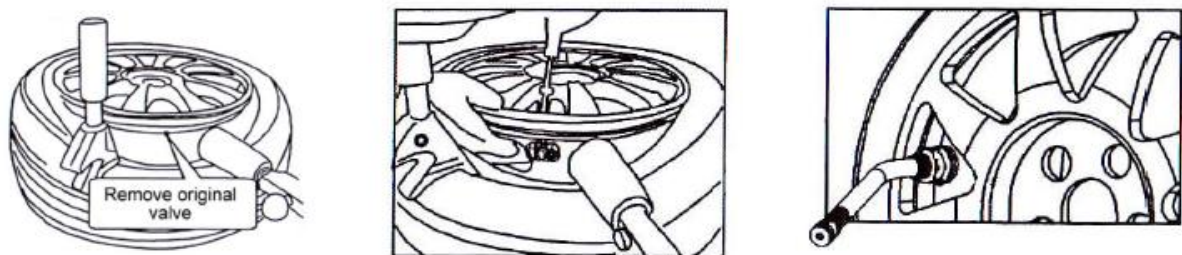
fig.4.6. Valve sensor installation
