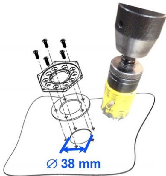
Fig. 7. Opening for sensor installation
