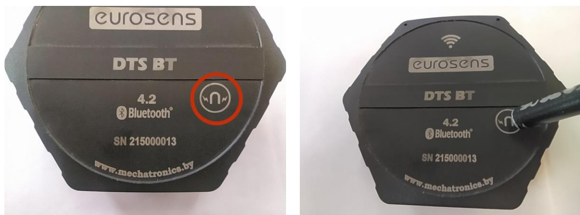
Fig. 5.3. Switching the sensor to service mode
