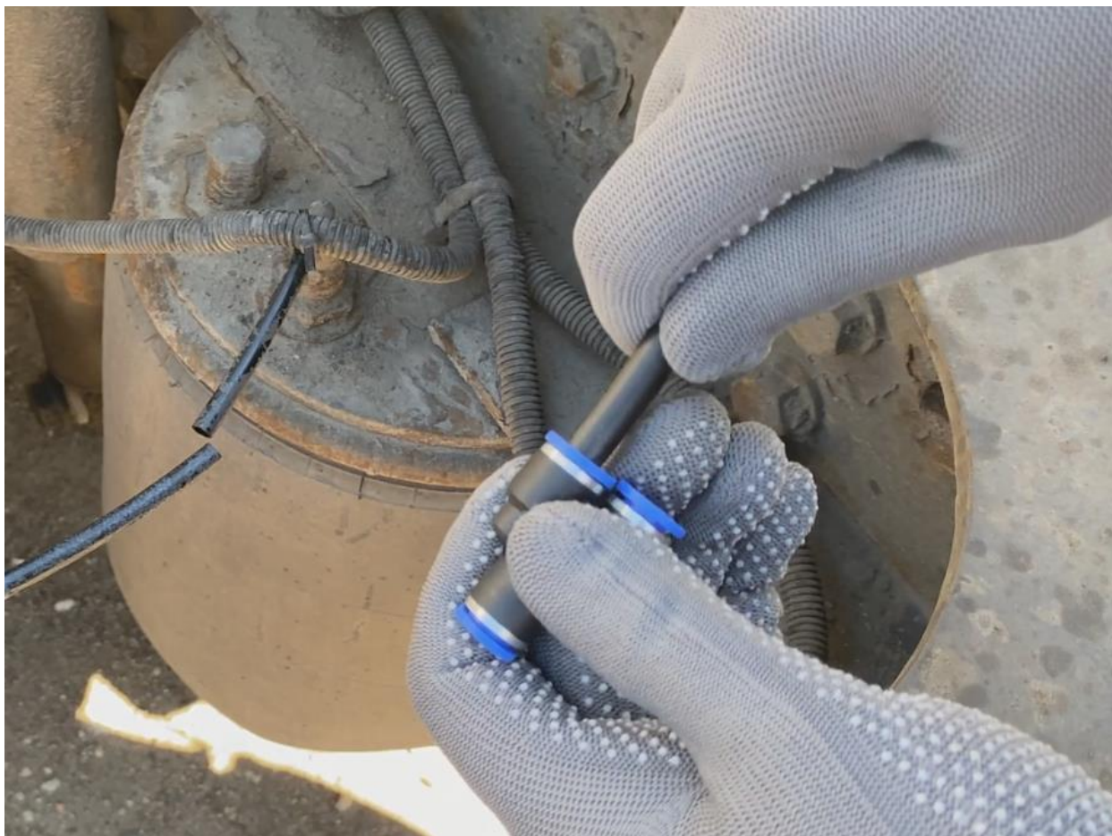
fig. 3.3. Installing pneumatic tube into connector
