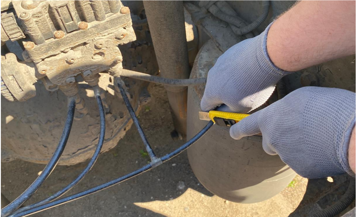
fig. 3.2. Cutting pneumatic line
