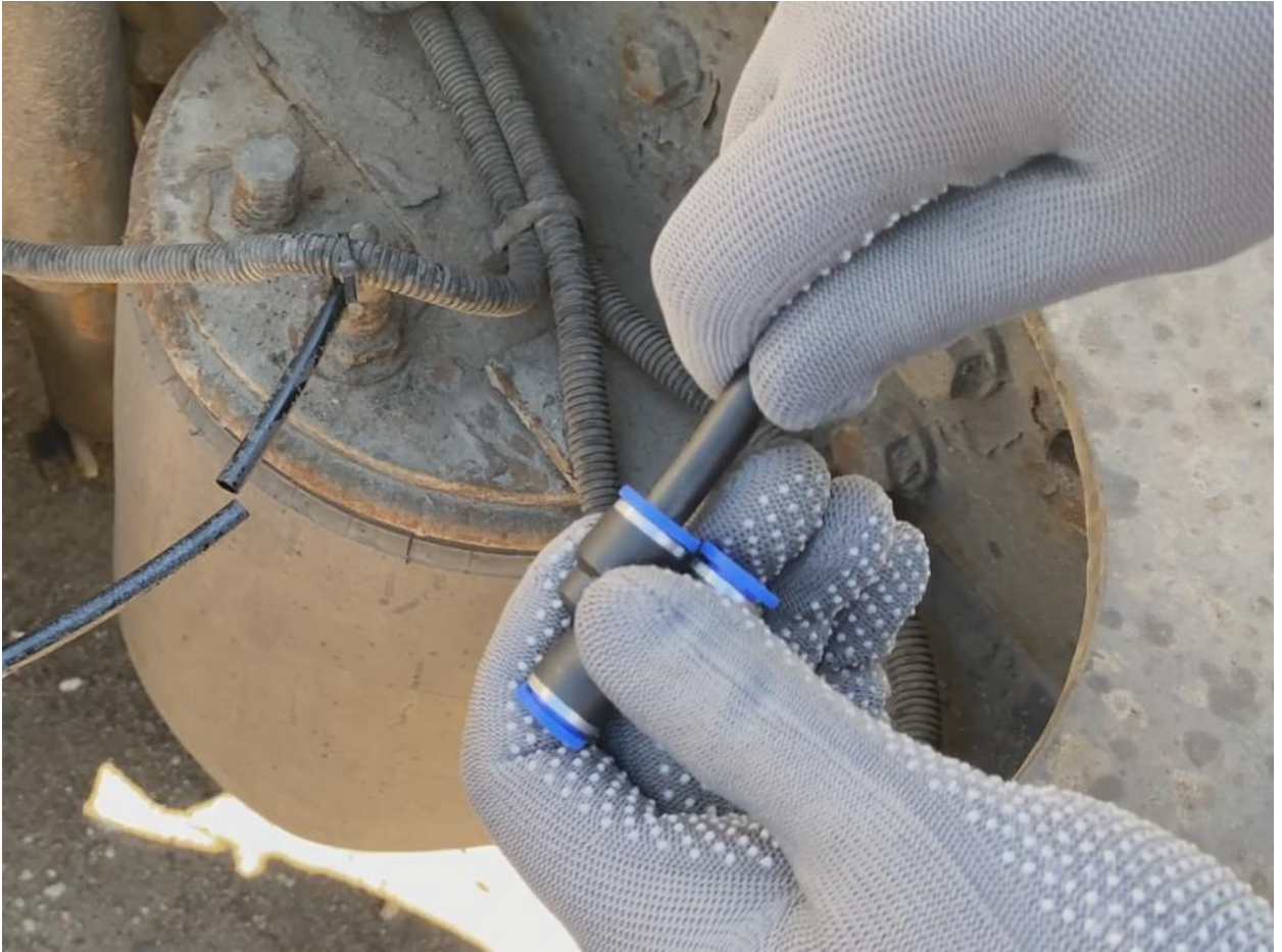
fig. 3.3. Installing pneumatic tube into connector
