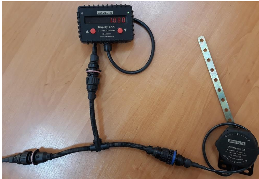
fig. 4.15. Display connection with Euosens DDS A sensor. Mode “Difference 02”
