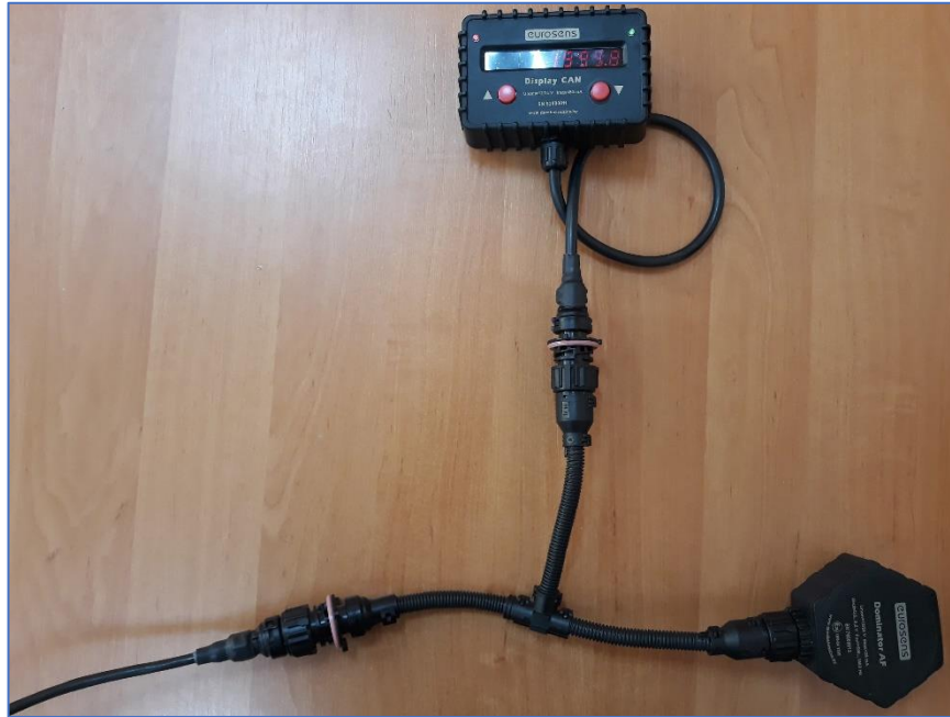
fig. 4.19. Display connected with fuel level sensor by analog interface
