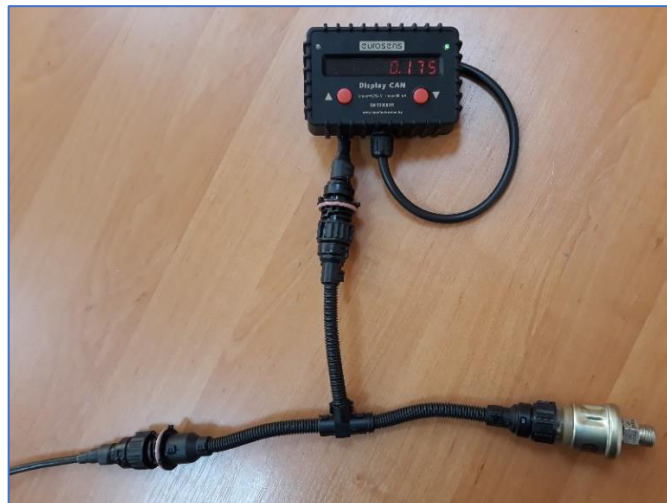
Fig. 4.11. Display connection with analog pressure sensor. Mode "Difference 01"
