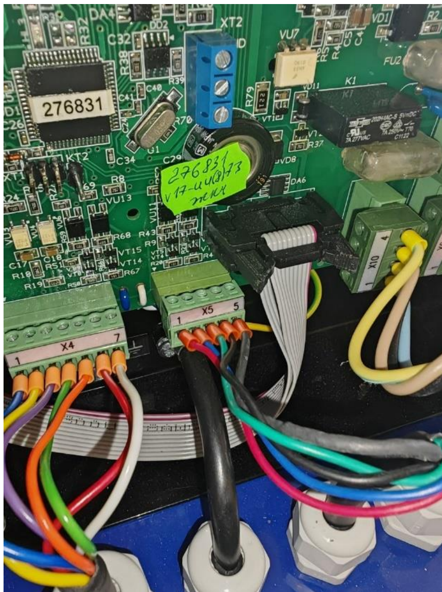
Fig. 7. Before connecting the reader (X5 connector: red wire +5 V, blue signal 1, green signal 2, black GND-, gray protective shielding).
