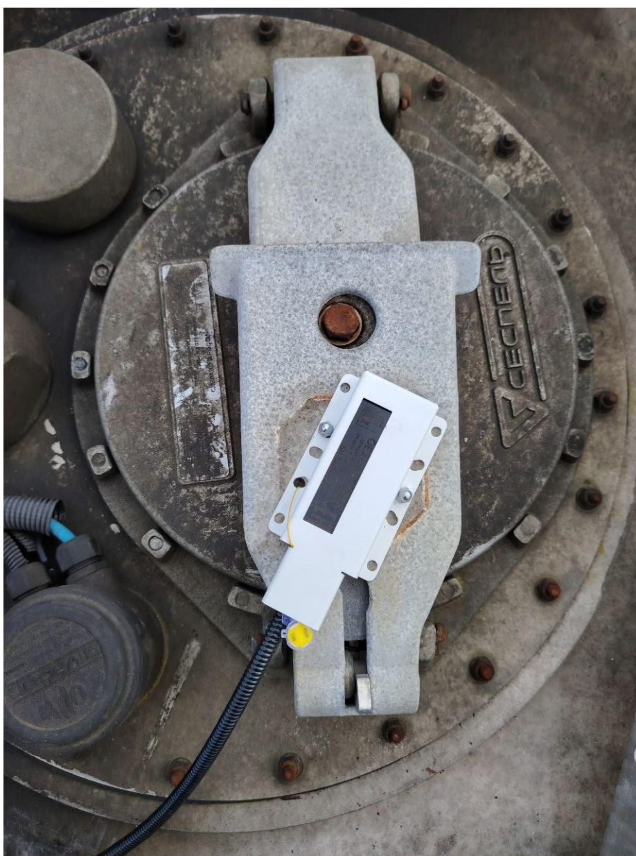
fig. 3.1. Using eurosens Degree on fuel tanker
