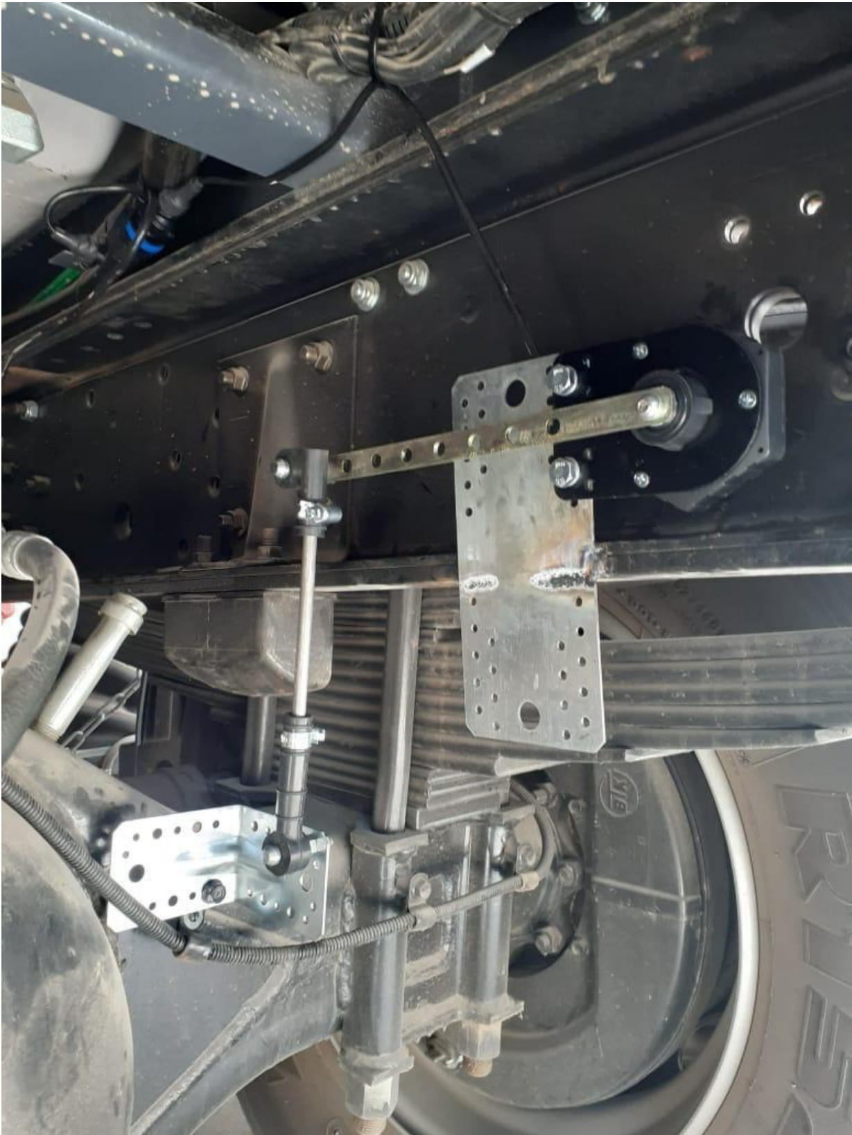
fig. 3.7. Sensor installation on front axle
