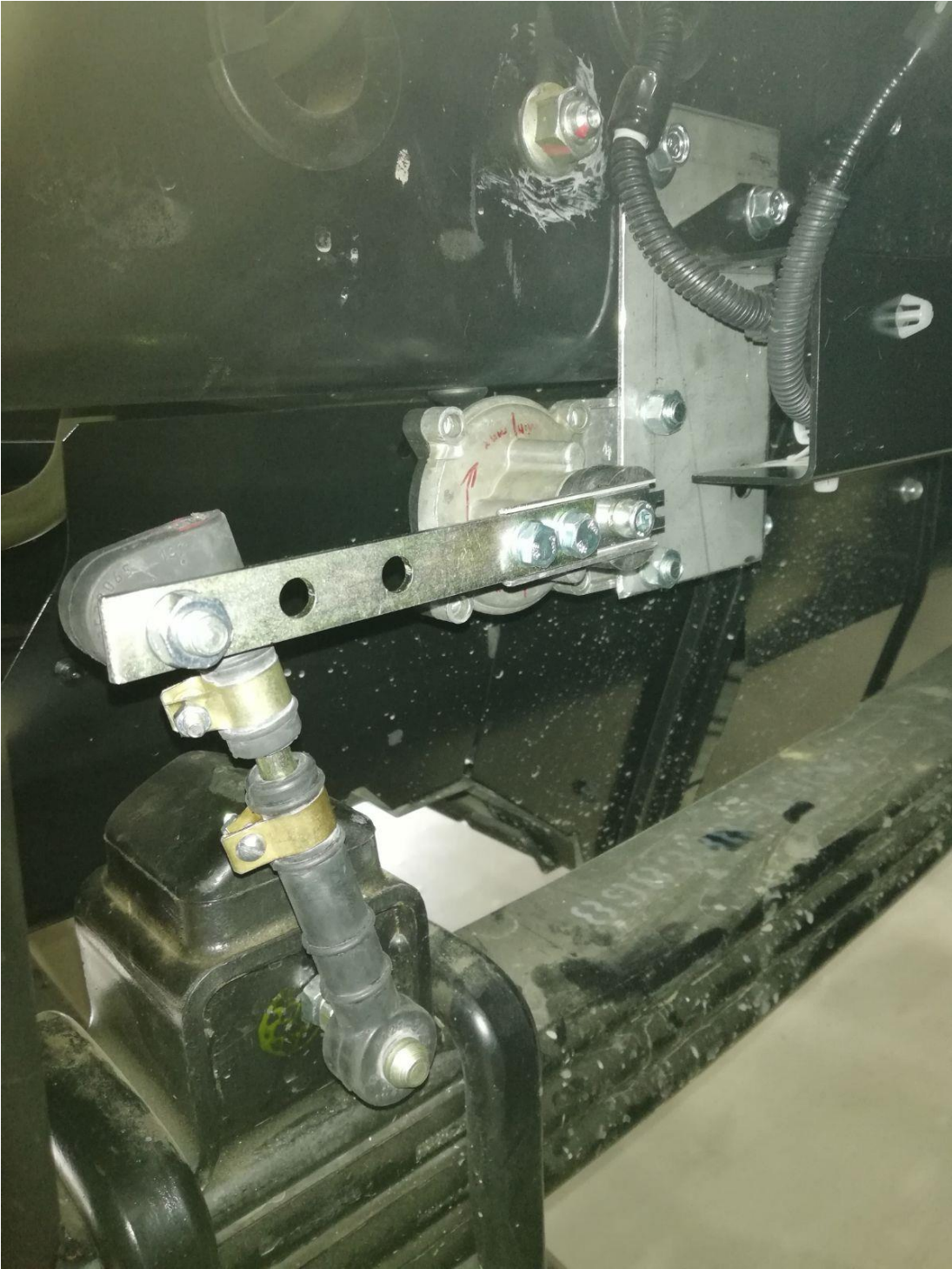
fig. 3.5. Sensor installation on front axle
