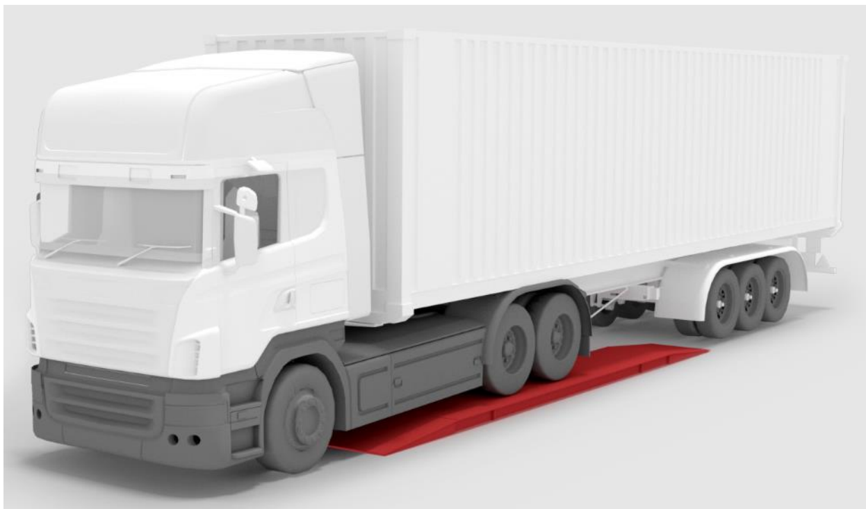
Fig. VIII. 2. Calibration of the rear axles of the truck
