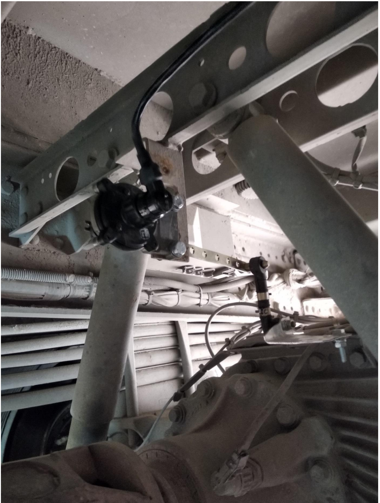
fig. 3.6. Sensor installation on front axle
