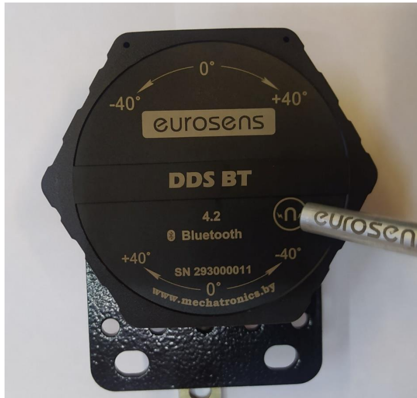
Fig. 5.7 How to activate the sensor
