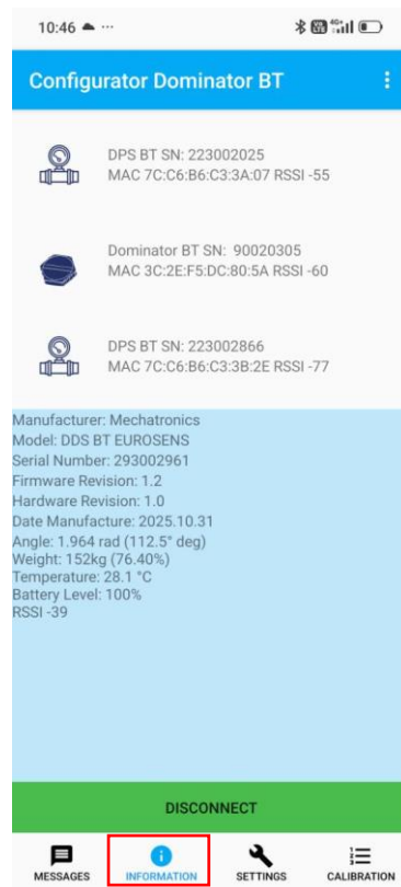
Fig. 5.9 Sensor information after connection
