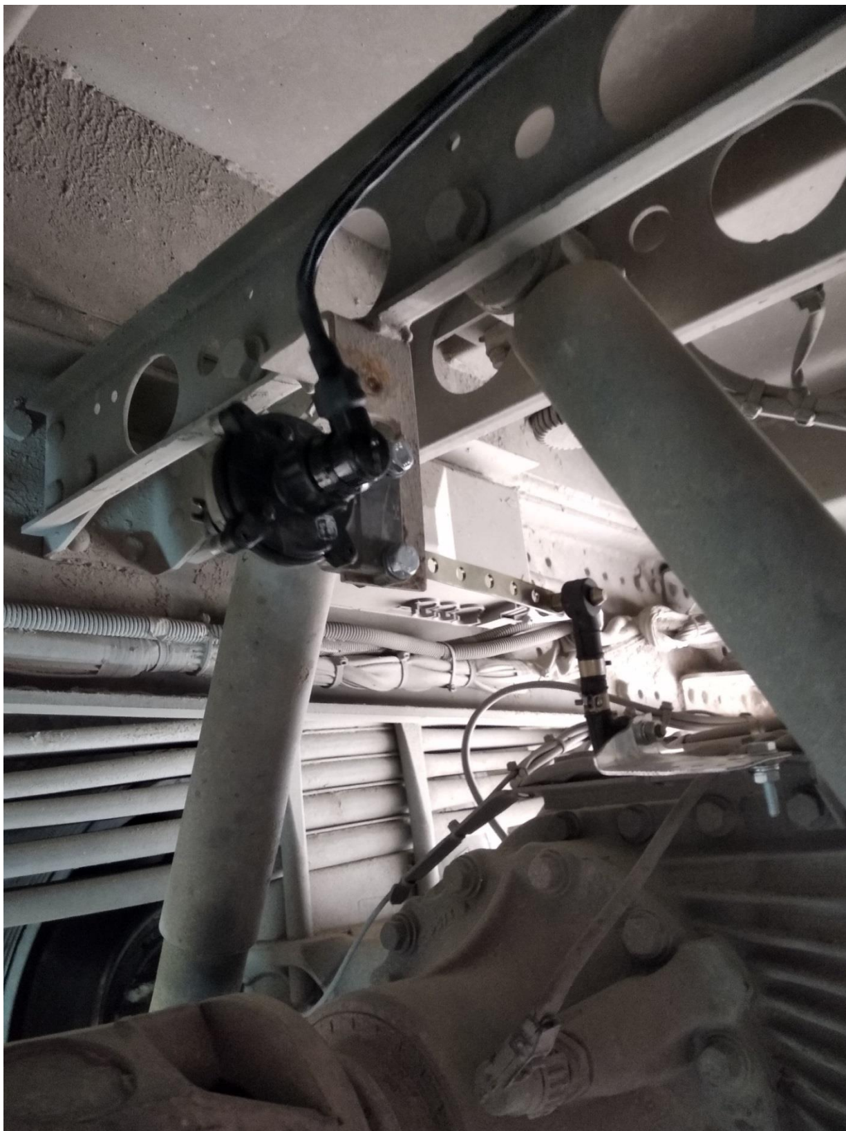
fig. 3.6. Sensor installation on front axle
