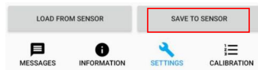
Fig. 6.3 Saving sensor configuration
