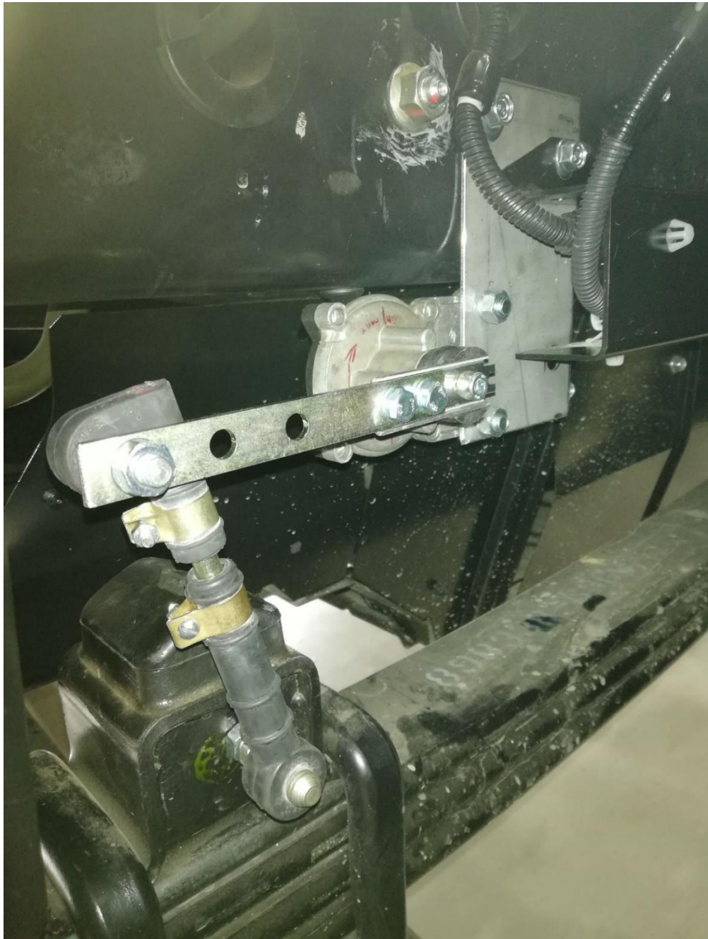
fig. 3.5. Sensor installation on front axle
